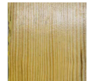
Varnish based on benchmark binder after aging test
