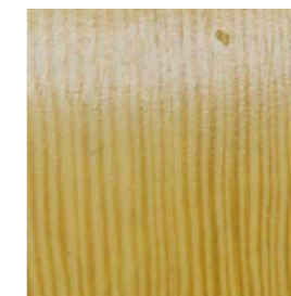
Varnish based on Synexil® AW 90CX after aging test
